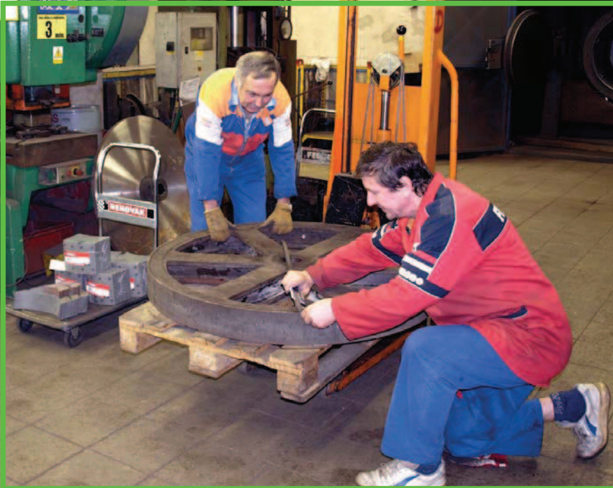
CONICAL CLUTCH D380xD365x6 SWR
