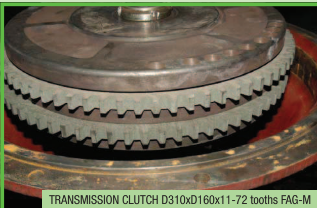
FRICTION PLATES D310xD160x11-72 toothes - FAG-M
